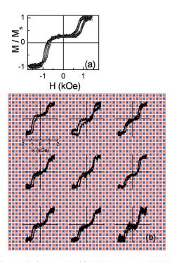
FIG. 2. (Color online) Protocol II. (a) MOKE loop at T=20 K illuminating the whole sample after cooling from room temperature at intermediate  $H_{\rm FC}$ =1 kOe. (b) Spatially resolved MOKE loops at different positions. Illustrated color-coded background as in Fig. 1.
