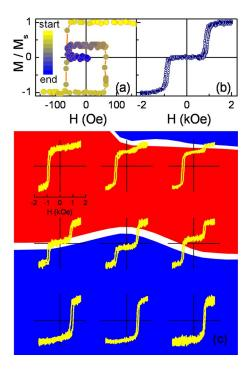
FIG. 1. (Color online) Protocol I. (a) Ni layer demagnetization at room temperature. (b) MOKE hysteresis loop at  $T=20\,$  K illuminating the whole sample after cooling at the remanence set in (a). (c) Spatially resolved MOKE loops at nine positions. Color-coded background: red, domains yielding negative EB; blue, domains yielding positive EB; white, domain walls between opposite domains.
