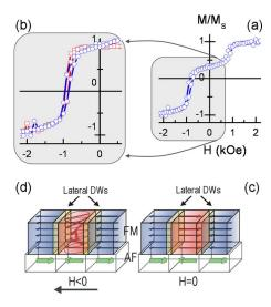
FIG. 3. (Color online) (a) DHL for intermediate  $H_{\rm FC}=1$  kOe. (b) Comparison between a *single loop* (low  $H_{\rm FC}=0.5$  kOe) (squares) and the rescaled *negative-biased subloop* from (a) (circles). Both loops were measured by SQUID at 10 K. (c) Illustrated spin configuration at H=0 and (d) H<0. Blue (left and right) and red (middle) domains yield positive and negative EB, respectively.
